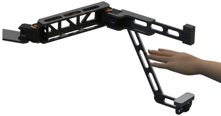
Figure 2: Kinematically optimized robot arm for additive manufacturing onto human anatomy [5]
